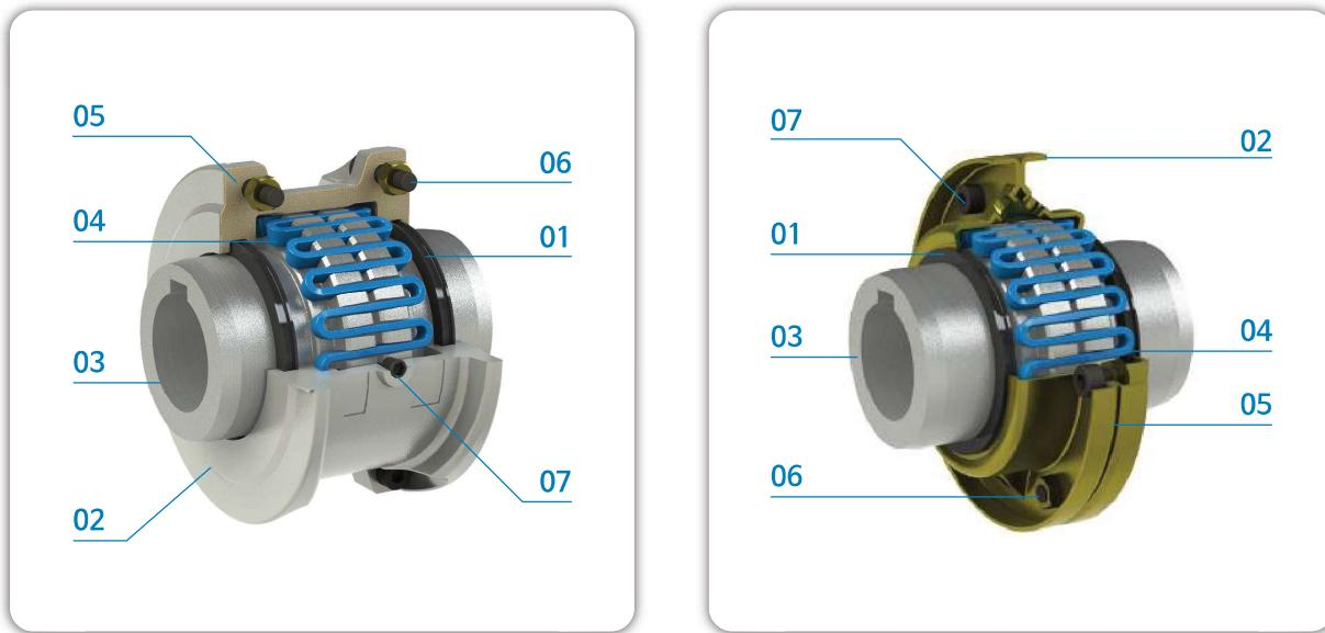
PART    01 Oil Seal    02 Cover    03 Hub    04 Grid    05 Gasket    06 Bolt    07 Lube Plug
